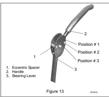
1. Remove the spacer, handle, and eccentric spacer from the steering lever.
